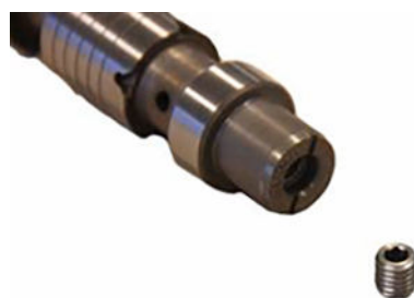
Dismantled directional spool (25) and orifice (26)
