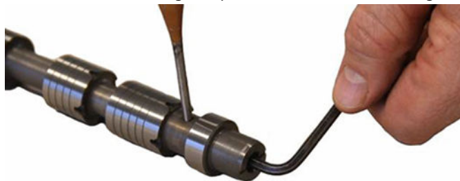
Dismantled directional spool (25) and orifice (26)
