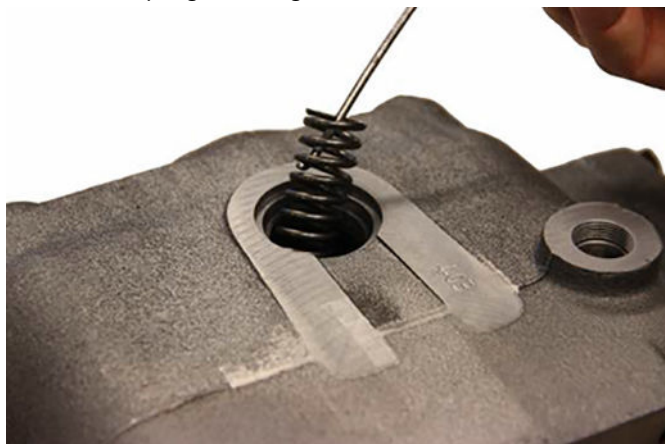
Dismantled counter pressure valve
