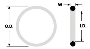
O-rings are round mechanical seals that keep gas or liquid from passing through an opening. Over time, these seals may wear out and require replacement. If you are planning to replace an o-ring, a good fit is critical. Also remember o-rings are measured in millimetres (mm).
