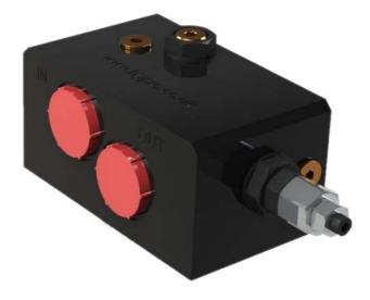
This special unloading inlet cover maintains 60lpm to the valve regardless of the inlet flow up to a maximum of 100lpm. Excess flow is returned to tank via the outlet port.
