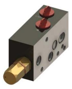
Options are available to have the outlet flow from both sides of the assembly combined into one outlet (MI) or as 2 separate outlets if the combined return flow is greater than 60 lpm (MIT).
